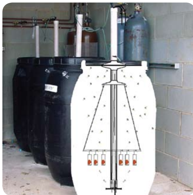
Figure 1 - Schematic cross-section of the anoxic and anoxic-reducing drums.
