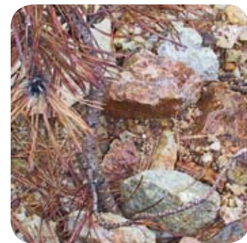
Growth trials within one of the Gilt Edge Mine drums containing a waste rock and Acid B™ reagent mixture.
