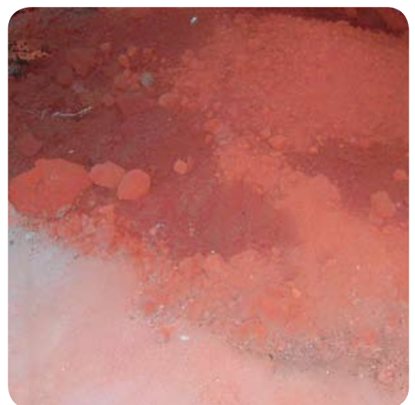
Electroplating waste treated with ElectroBind™ reagent and ready to be disposed to landfill.
