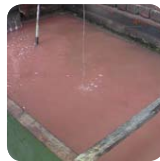
Addition of ElectroBind™ reagent to the mixing tank
