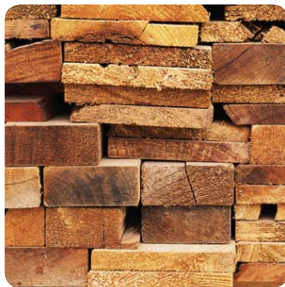
With the CCA treatment process, copper and arsenic protects timber from insect and fungal degradation. Chromium seals the copper and arsenic into the timber.
