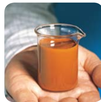
ViroBond™ Reagent immobilises heavy metals into an insoluble, non-hazardous sediment.
