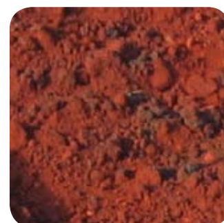
Treated soil after ViroBond™ reagent addition
