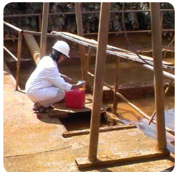
These concrete channels were the input to the lime treatment plant in Baia Mare. Two mega litres of AMD water was transferred from this plant to a containment dam that was used to test the Acid B Extra™ reagent.
