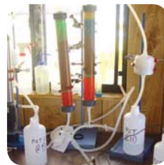
Conducting ViroFilter™ Passive Treatment trials at Gilt Edge Mine. The cells that gave the results overleaf in Table 4 were much larger - these small cells were subsequently used to help understand the limits of the method.
