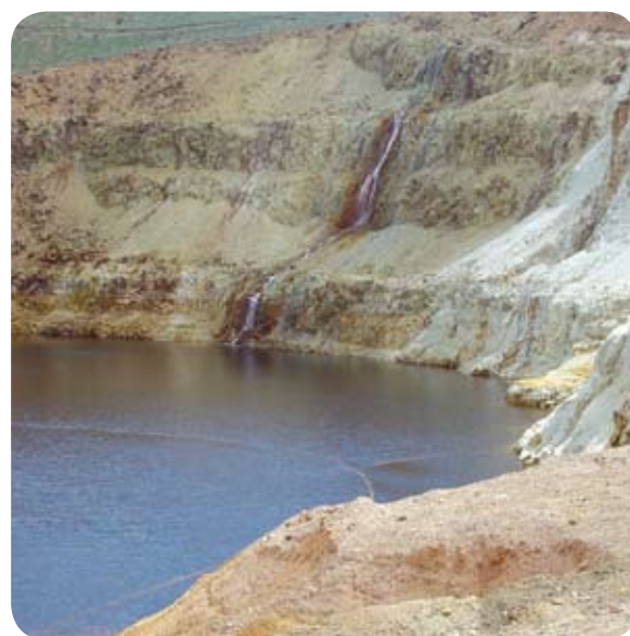
One of the contaminated pit lakes - with flowing ARD visible to the right.
