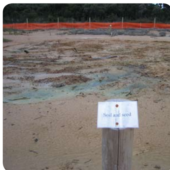
Photograph showing the condition of of the 100m2 lime and fertiliser treated plot 12 months after treatment; note pools of salt water that have accumulated on the treated area as a result of seawater inundation.
