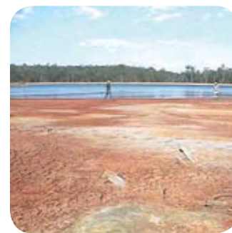
This photo shows the exposed area of tailings where grass was grown during this study. The photo also shows the very thin layer of the Acid B™ reagent that remained after the water had been released from the tailings dam.
