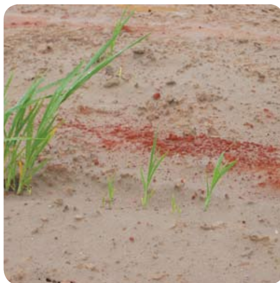
The germination of grass in the acid tailings after mixing the Acid B™ reagent residues, remaining after water treatment, into the exposed tailings beach.
