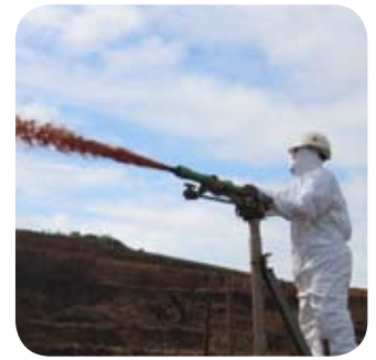
ViroMine™ Technology Acid B Extra™ reagent is designed to treat sulphidic waste rock and soil.
