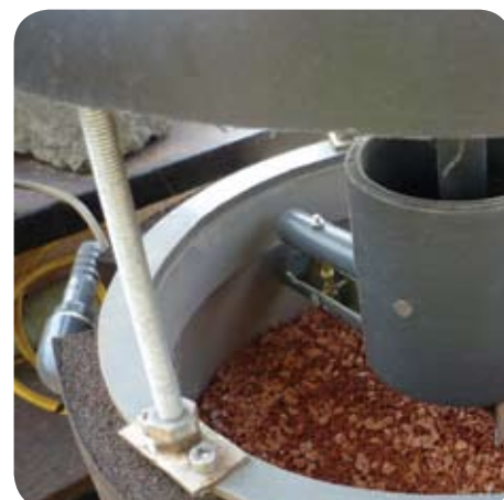
Influent head of the ViroFlow™ Technology filter system
