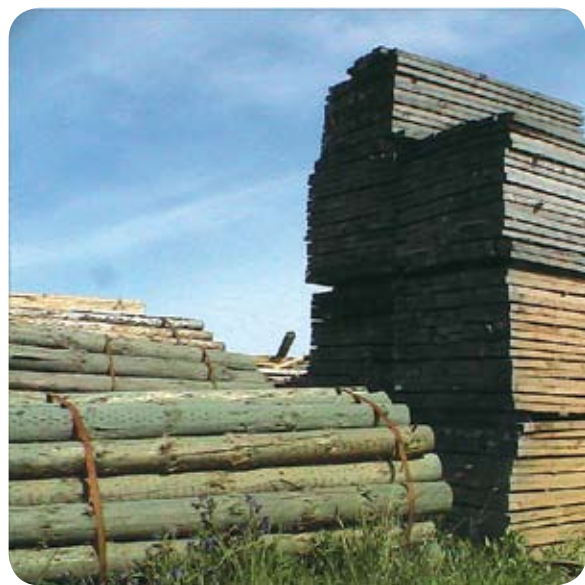
Leachate from stored timber is contaminated with heavy metals.
