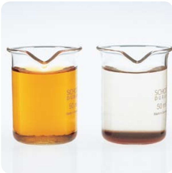
Tannery wastewater before and after treatment – chromium levels and odour were greatly reduced
