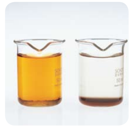
Acid Rock Drainage before and after ViroMine™ Technology treatment.
