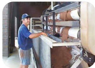
Biocake treated with ViroSewage™ Technology had virtually no odour and had higher percent solids than untreated material.
