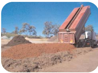
ViroSewage™ Technology treated biosolids being mixed with green waste.
