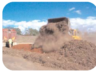
ViroSewage™ Technology treated biosolids being mixed with green waste.
