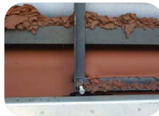
Biocake treated with ViroSewage™ Technology had virtually no odour and had higher percent solids than untreated material.
